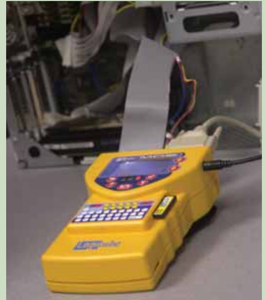
Equipment in the Florida Law Enforcement Electronic Evidence Team lab allows investigators to copy and analyze data from seized computer hard drives.
